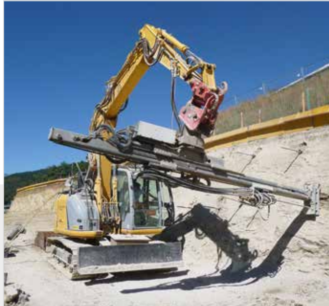
Exact alignment of the drilling rig at the drilling position.
