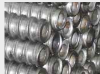
Stainless steel - INOX Non-corroding stainless steel (grade 1.4462)
