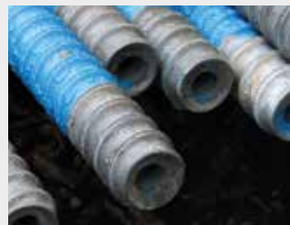
DUPLEX protection Hot-dip galvanizing + powder coating + epoxy powder coating to DIN 55633
