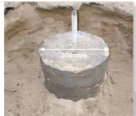
Grout body injected into soft sand with high pressure (TITAN 40/16 micropile with Ø 110 mm clay bit and carbide nozzle)
