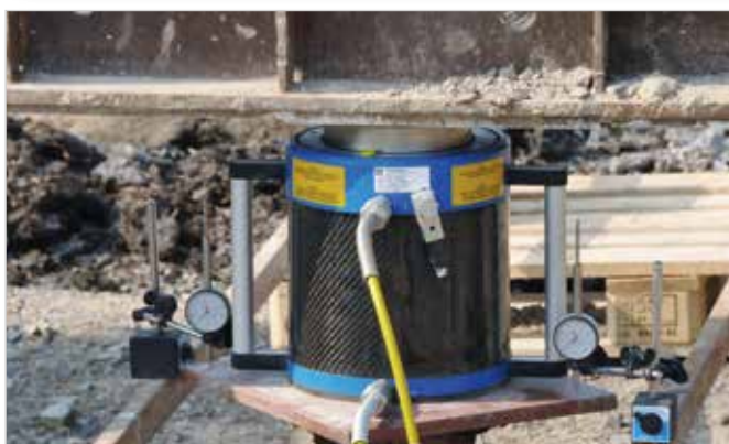
Compression loading test on micropiles in soil with a risk of buckling.
